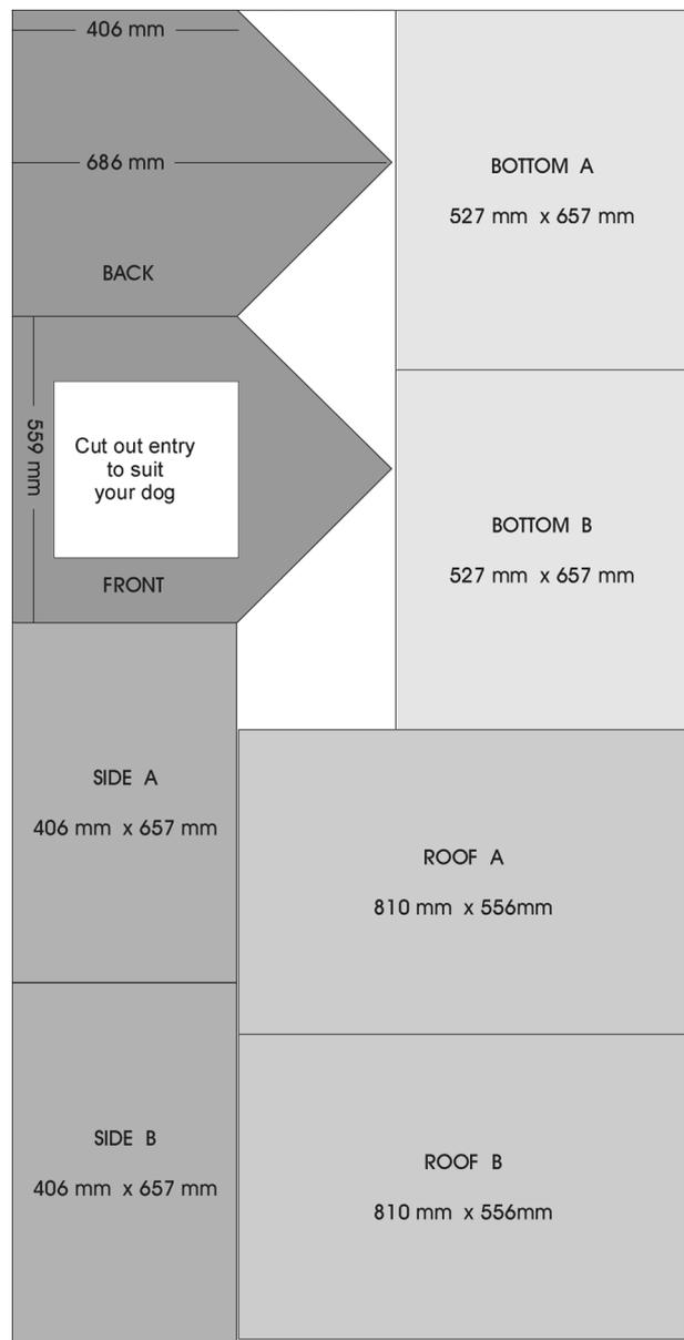
Cutting guide using 2440 mm x 1220 mm x 16 mm ply
